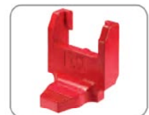
One-piece cast iron safety toe for one-hand operation. A tothing in the front region avoids slipping off the load. Very high safety margin. A peg on the back secures correct insertion.
