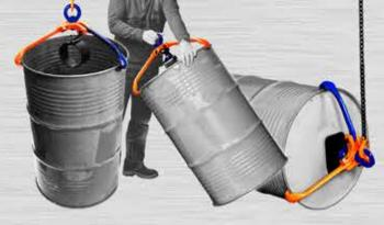
Operational in situations on the open sea, on uneven ground or flatlaying drums covered in oil or grease.
